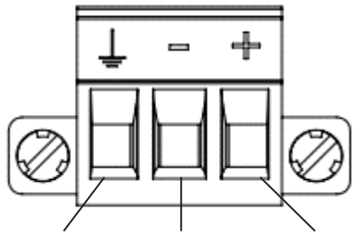
FG (functional grounding terminal) DC input terminal (-V) DC input terminal (+V)
