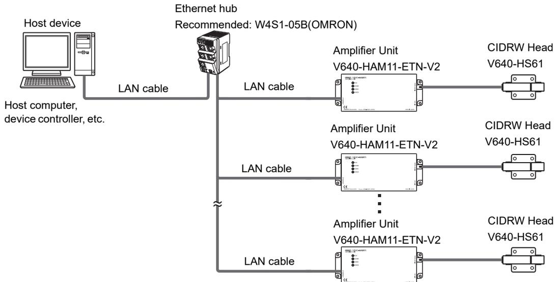
The Amplifier Unit controls the CIDRW Head.
