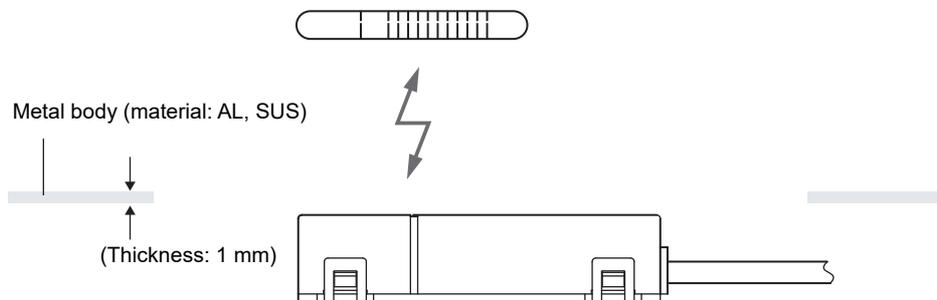
However, ensure the distances indicated below between the CIDRW Head and the metal body. If you do not ensure these distances the communications distance will be substantially shortened.
