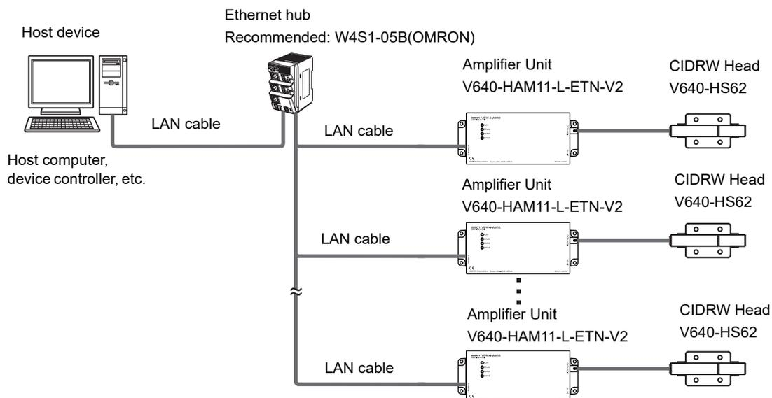
The Amplifier Unit controls the CIDRW Head.
