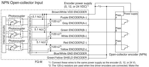
software settings to turn OFF the switches that are connected to the 120-Ω resistors when open-collector encoders are connected.
