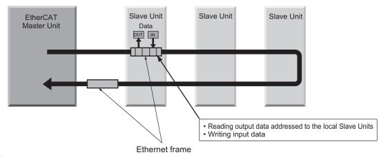
It is the " fercar telegram" stored directly in an Ethernet frame that exchanges data regularly between the EtherCAT Master Unit and Slave Units.
