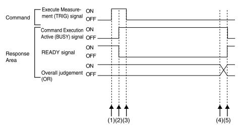
(1) Measurement starts when the TRIG signal turns ON while the BUSY signal is OFF.
