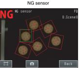
Automatically changes to the display for any Sensor with an NG result.
