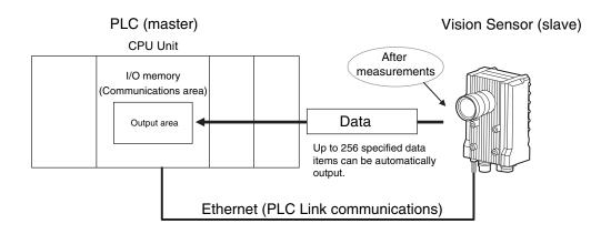
You must specify in advance the data to output after measurements. You must also specify in advance the Output Area in I/O memory to store the data in the PLC. After a single measurement or continuous measurements, the data is automatically stored in the Output Area of the PLC via Ethernet.
