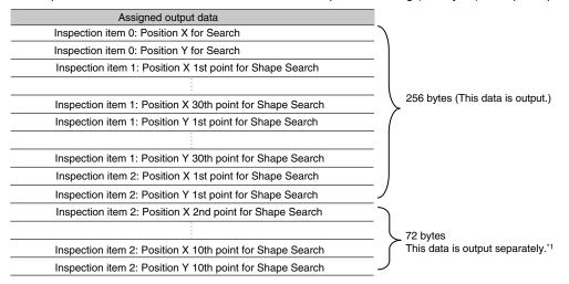
\*1 If the size of the specified output data exceeds the set value of the data output size setting, the data is output separately as shown below.
