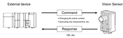
The external device sends a command as an ASCII string (e.g., "MEASURE" for a single measurement). The Vision Sensor then returns a response such as "OK", "NG", or some value.
