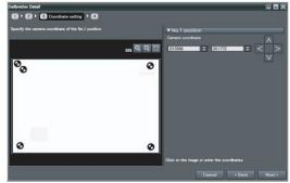
5 Enter the X and Y coordinates after calibration in the [Coordinates of control device] fields.
