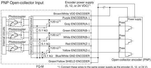
\*1: Connect these wires to the same power supply as the encoder (5, 12, or 24 V).
