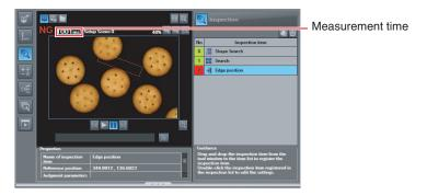
The measurement time is the time taken from when a trigger is input until when all measurement processes are executed.
