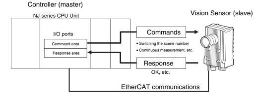
After you write a control command to an I/O port, such as Vision Command, you can turn ON the Control Command Execution (EXE) Bit to send the control command to the Vision Sensor via EtherCAT. The Vision Sensor executes the control command and sends a response back to the Controller via EtherCAT. The Controller stores the response in an I/O port, such as Vision Response.
