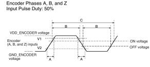
\* The graph shows the input waveform for a PNP encoder.
