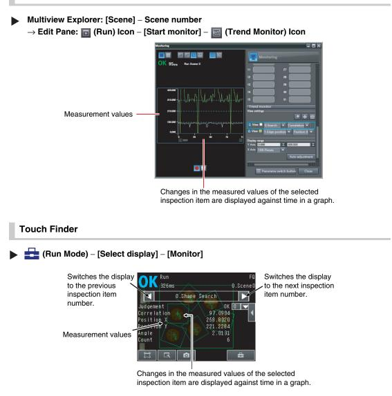
If there is a high load on the Sensor for measurement processing, display data can sometimes be omitted from the Trend Monitor. To prevent display data omissions, set the BUSY signal output timing to [Result display]. If the Sensor is being controlled over a PLC link, execute the next command only after confirming that the BUSY signal from the Sensor is OFF.
