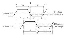
\* The graph shows the input waveform for a PNP encoder.
