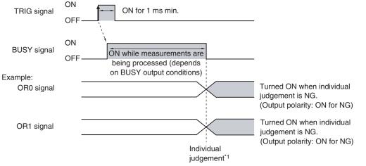
\*1: The timing for updating the OR signal is when the measurement results are finalized, regardless of the output settings of the BUSY signal (BUSY output conditions).
