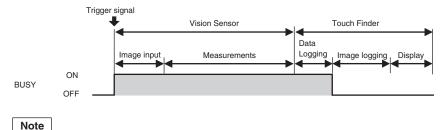
• File logging cannot be used when performing continuous measurements.
