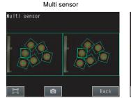
Displays the measurement results of all connected Sensors. Green display: OK, Red display: NG
