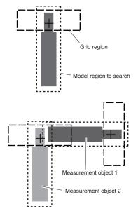
**3** Only the search results for workpieces that have been determined as being able to grip with gripping areas at or above the grip area level are output.
