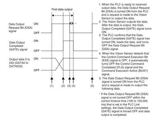
Data Output after Measurements When Handshaking Is Disabled
