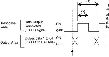
The data is output according to the set output cycle (1) and output time (2).
