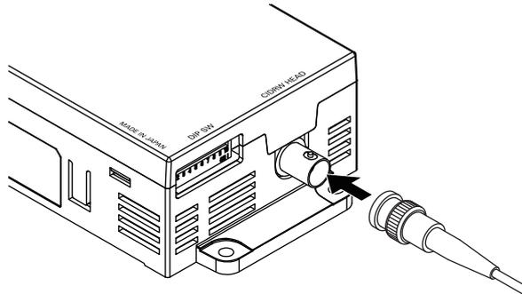
2. After inserting the connector fully home, turn the fixed part clockwise to lock it.
