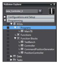
The **Controller** block whose code is outputted by the Simulink PLC Coder and its internal blocks **CommandPositionGenerator** and **PositionController** are imported as function blocks of Sysmac Studio.
