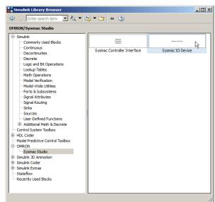
Double-click the Sysmac IO Device block added in Step 10. The setting dialog box for selecting a device in the Sysmac Studio project is displayed.
