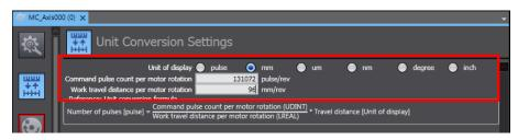
5 Make the Operation Settings according to the mechanical configuration.
