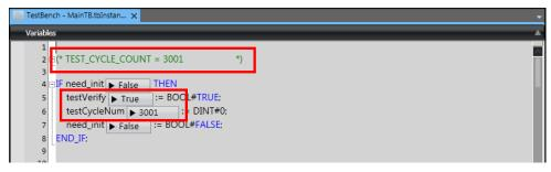
You can confirm that calculation accuracy of the output data is the same level as the Simulink (within the acceptable error range) if *testVerify* is True.
