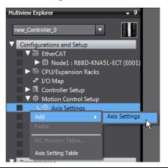
2 Double-click MC\_Axis000(0) (Axis 0) that was added under Motion Control Setup - Axis Settings in the Multiview Explorer to display the axis parameter setting view.
