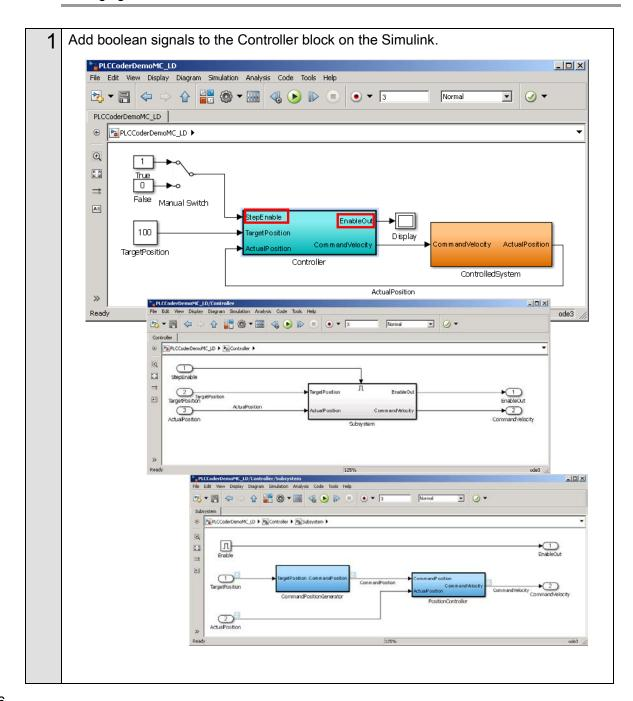
When the code is imported to the Sysmac Studio, the BOOL variables are added as shown below.
