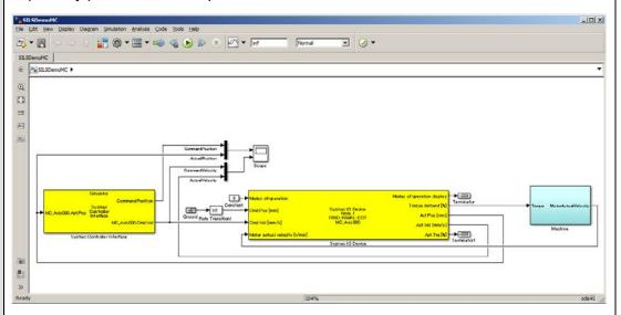
7 Double-click the Sysmac Controller Interface block. The setting dialog box for exchanging the data between Simulink and Sysmac Studio is displayed.
