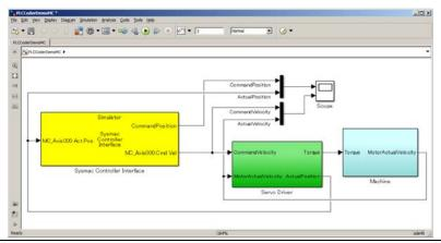
Select the Sysmac IO Device block from the Simulink Library Browser and add it to the Simulink model.
