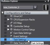
2 Set the task period to 1 ms in the Task Settings View on the Sysmac Studio so that the period matches the sampling time of the Controller on the Simulink.
