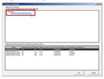
Select *R88M-K10030T* from the list of servomotors that can be connected to the Servo Drive selected in Step 12.
