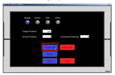
Click the **Home** Button on the Test Window for the Programmable Terminal. The axis is returned to the home.
