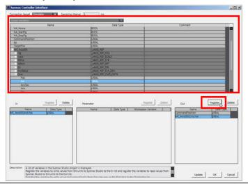
7 Select *Kp* from the list of variables in the Sysmac Studio project and click the **Register** Button for the Parameter list to pass the values from Simulink to Sysmac Studio only in the first step,
