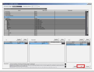
**9** Delete the Controller block and replace it with the Sysmac Controller Interface block that you added.
