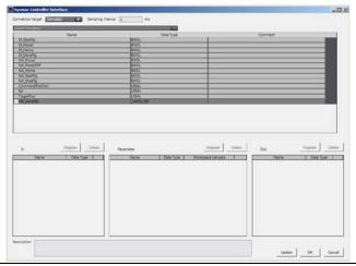
4 Select *MC\_Axis000.Act.Pos* from the list of variables in the Sysmac Studio project and click the **Register** Button for the In list to pass the actual current position calculated by the Simulink to the Sysmac Studio's Simulator.
