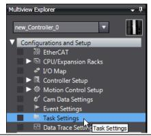
4 Set the task period to 1ms in the Task Settings View on the Sysmac Studio so that the period matches the sampling time of the Controller on the Simulink.
