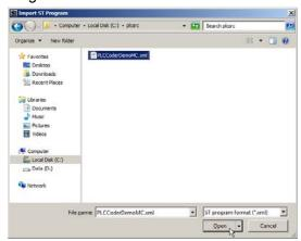
The data is imported and the programs, functions, function blocks, data types, and global variables in the XML file are added to the project of Sysmac Studio.
