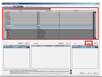
Select MC\_Axis000.Cmd.Vel from the list of variables in the Sysmac Studio project and click the **Register** Button for the Out list to pass the velocity command value for the Servo Drive calculated by the Sysmac Studio's Simulator to the Simulink.
