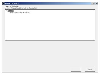
12 Select the Servo Drive whose node address is *1* from the EtherCAT network configuration in the Sysmac Studio project.
