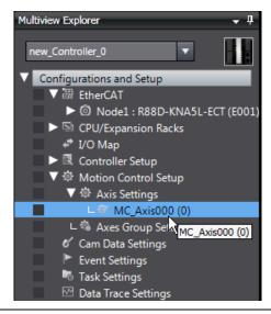
3 | Make the Axis Basic Settings as shown below to assign the Servo Drive to the axis.
