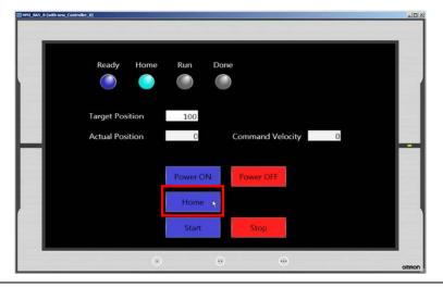
Click the **Start** Button on the Test Window for the Programmable Terminal. The axis starts moving to the Target Position and the **Run** Lamp is lit. The Actual Position value and Command Velocity value change. When the movement is completed, the **Done** Lamp is lit.
