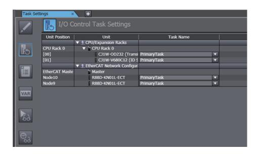
3 Select the task that should perform I/O refreshing for the registered Unit from the list.
