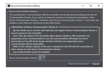
In the **Secure Communications Setting** Dialog Box, select a **Secure Communication Version** and click the **Transfer to controller** Button.
