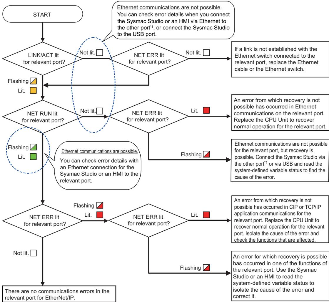
\*1. You can connect the Sysmac Studio or an HMI to the other port to confirm error details only when Ethernet communications are possible for the other port.
