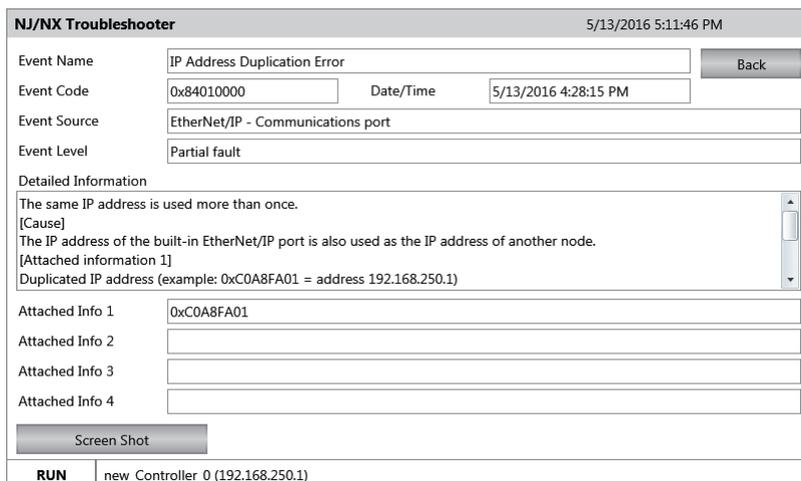
After you complete all of the correction steps for the current errors, click the **Error Reset** Button in the Controller Event List Screen to reset all of the current errors.
