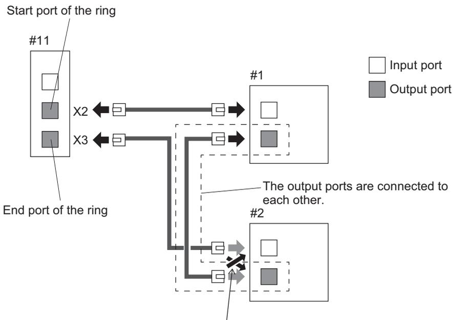
Between slaves in the ring topology connected to ports X2 and X3 of slave #11 described in the attached information, re-connect the cable whose ends are both connected to output ports to the input port in the next slave.
