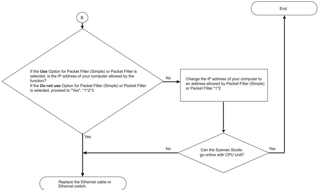
\*1 For details on Packet Filter (Simple) setting and Packet Filter setting, refer to the *NJ/NX-series CPU Unit Built-in EtherNet/IP Port User's Manual* (Cat. No. W506).
