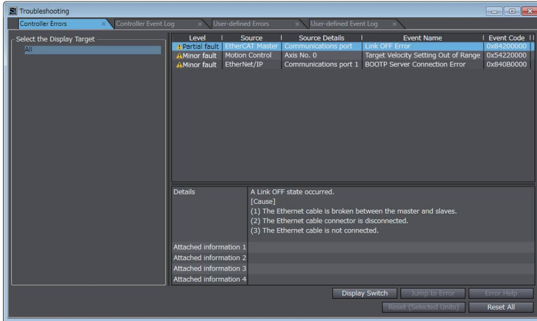
To eliminate the cause of the error, first select the item to perform from the Action and Correction list. When you select the appropriate step in the Action and Correction list, either the **Jump to Error** or **Error Help** Button is enabled, depending on the contents. In some cases, neither button will operate. Click the enabled button, and proceed with the displayed troubleshooting steps.
