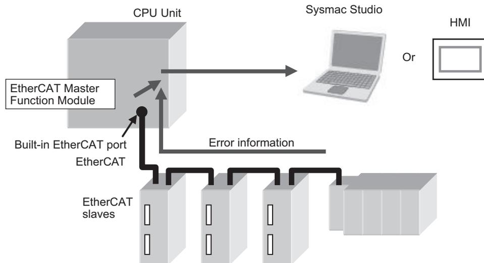
If an error occurs at the same time for more than one slave, only the error occurred for some slaves is registered among current errors or recorded in the event log as follows. When you clear a registered or recorded error on a slave, the error occurred on another slave may be registered or recorded. Make corrections repeatedly until the error is no longer registered or recorded.
