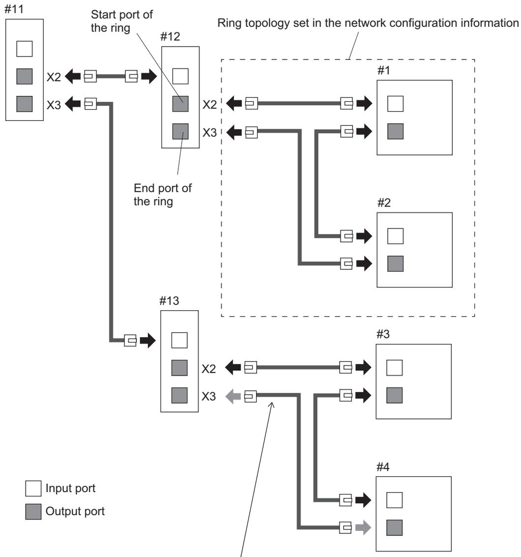
For the ring connections made to ports X2 and X3 of slave #13 not described in the attached information, remove the cable connected to X3 of the end port of the ring.
