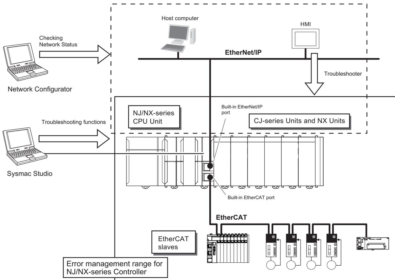
You can use the troubleshooting functions of the Sysmac Studio or the Troubleshooter on an HMI to quickly check for errors that have occurred and find corrections for them.
