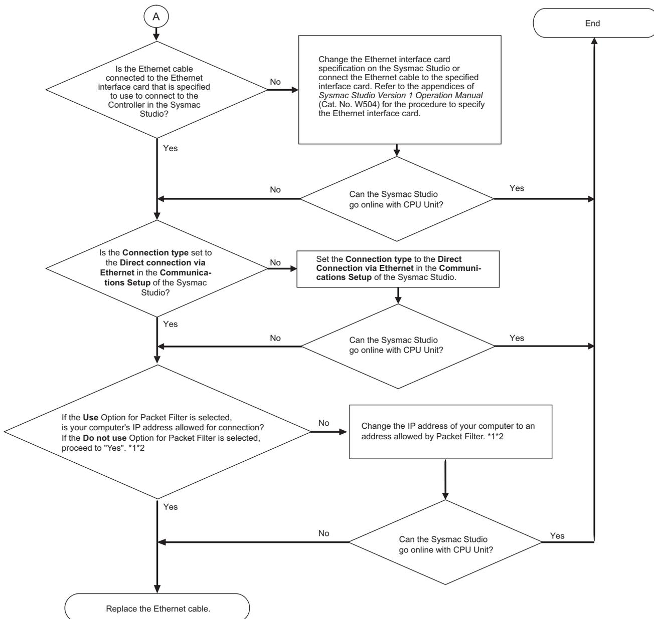
\*1 For details on Packet Filter (Simple) setting and Packet Filter setting, refer to the *NJ/NX-series CPU Unit Built-in EtherNet/IP Port User's Manual* (Cat. No. W506).
