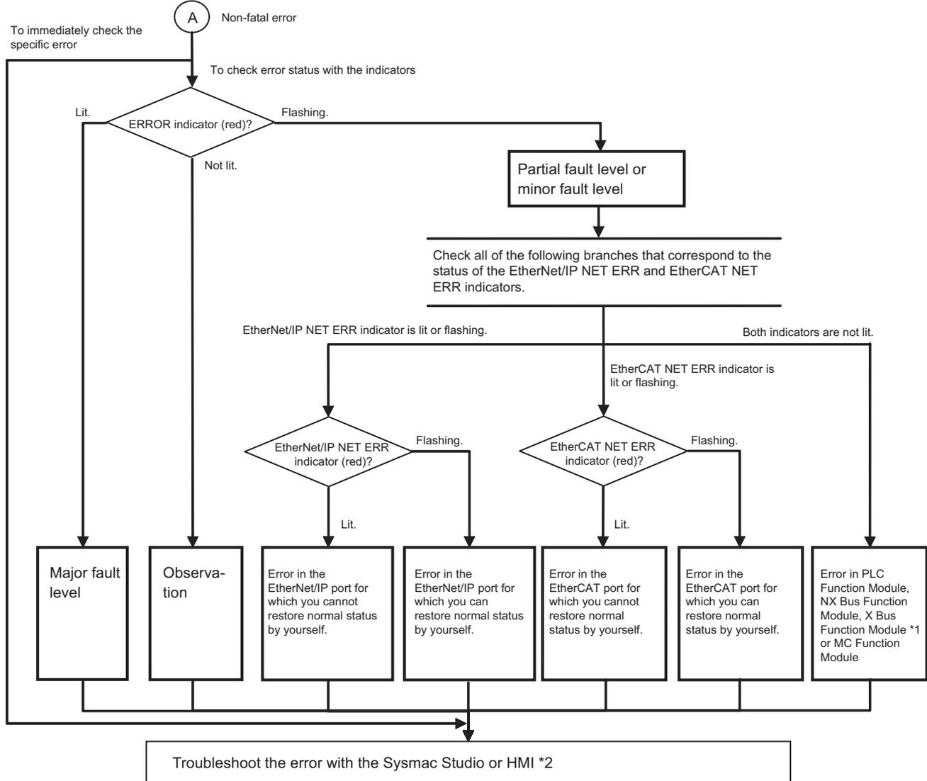
\*1. Refer to the 3-4 *Errors in the X Bus Function Module* on page 3-444 for information on X Bus errors. For information on the X Bus Unit errors, refer to *Troubleshooting* in the user's manual for each X Bus Unit.
