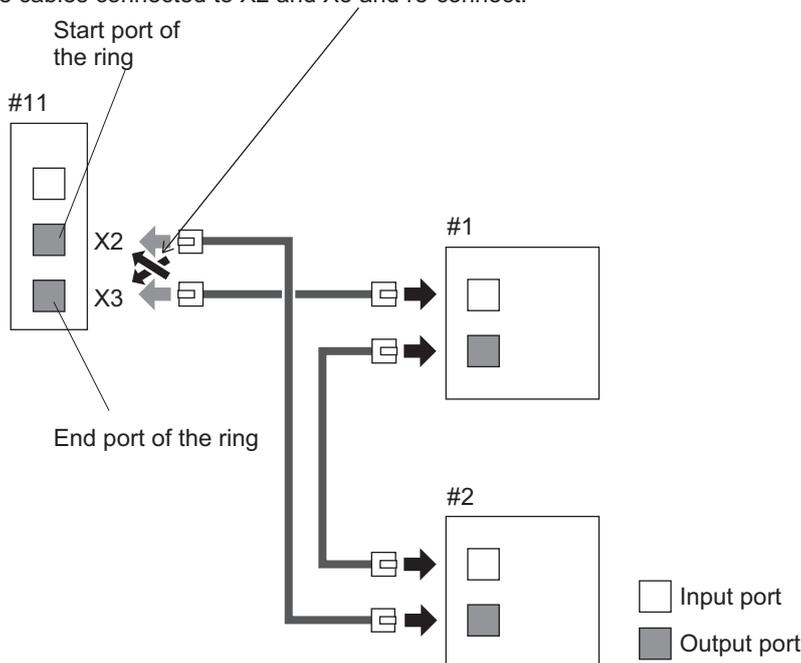
● **If the Subsequent Slave in the Ring Topology Is Connected to a Port That Is Not the Last Port on a Junction Slave in the Ring Topology**
