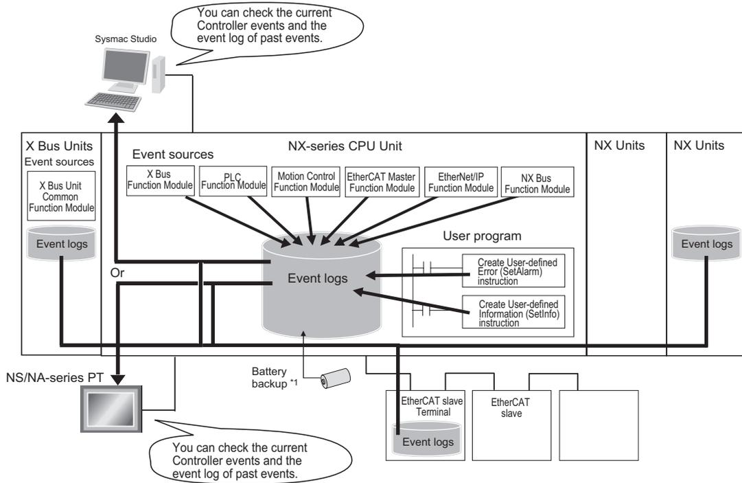
\*1. The event logs are saved in battery-backup memory in the NX701 CPU Unit.
