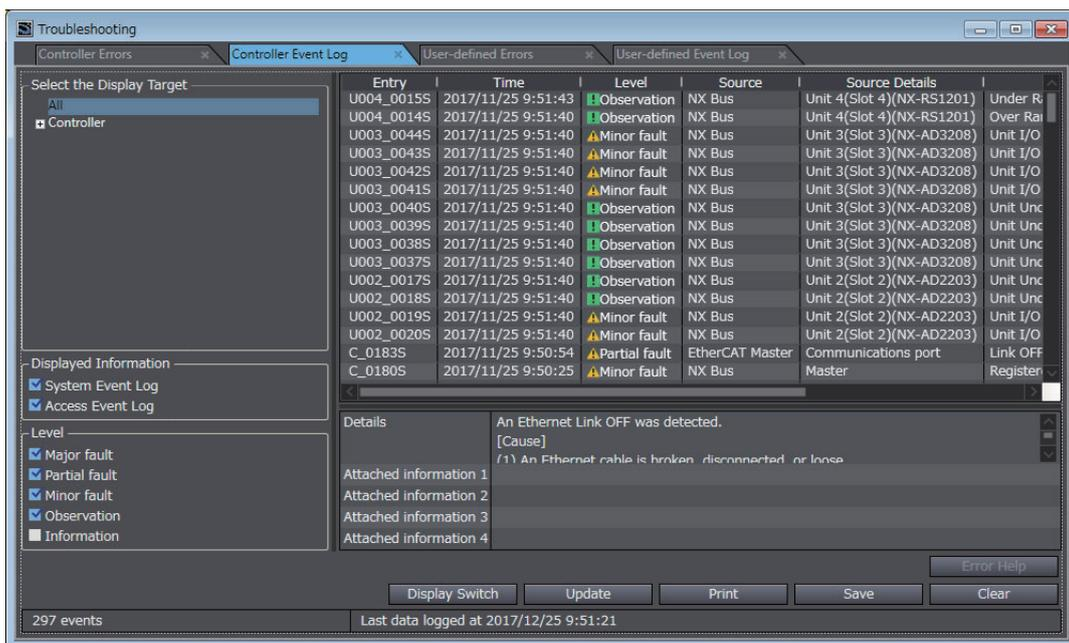
Error logs from CJ-series Special Units are displayed on the **Controller Event Log** Tab Page. Detailed information is not displayed. To check detailed information, use the event codes that are displayed and refer to the error codes that are given in the manual for the relevant Unit. The relationship between error codes and event codes is described in *Details on Controller Events (Errors and Information)* on page 1-15 under *1-3-1 Types of Non-fatal Errors* on page 1-12.
