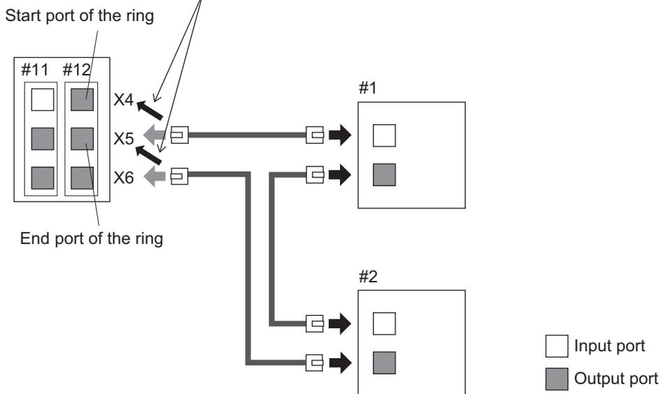
● **If the Wiring for the Start Port of the Ring and One for the End Port of the Ring Are Reversed on the Actual Network**
