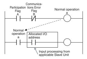
• The operation of the Participation Flags and Communications Error Flags depends on the status of pin 4 (REGS) on the CompoNet DIP switch on the front of the Gateway Unit.
