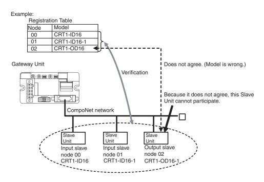
This function is enabled only in Registration Table Enable Mode, i.e., when pin 4 (REGS) is ON on the Gateway Unit when the power is turned ON and the registration table data is normal. It can be used in any communications mode.
