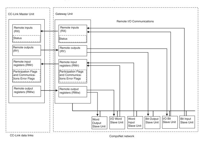
• The Slave Units on the CompoNet network are assigned to buffer memory in the CC-Link Master Unit as follows:
