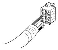
The communications connector is labeled with the terminal names. Align the colors of the communications wires with the terminal names on the connector to ensure that the wires are connected correctly.
