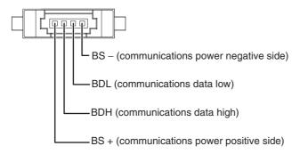
Note: BS – and BS + terminals output the communications power that is supplied from the power connector. (They also supply power to Slave Units and Repeater Units on the trunk line.)
