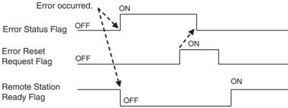
\*4 This flag turns ON when the power supply is turned ON or after resetting with the reset switch.
