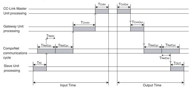
TCclin: CC-Link input delay TCcOut: CC-Link output delay
