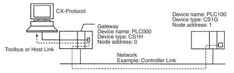
Note This type of connection is not supported for an NJ-series CPU Unit.
