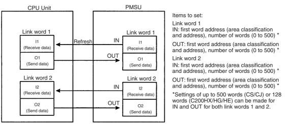
Creation of send messages and storage of receive messages is performed using the link word area.
