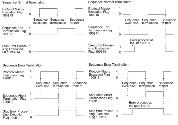
Note 1. The Step Error Processing Execution Flag is not a flag for the whole sequence, but a flag to determine whether the error process is executed at a step in the sequence. Therefore, as in the above example 2, if the consec-
