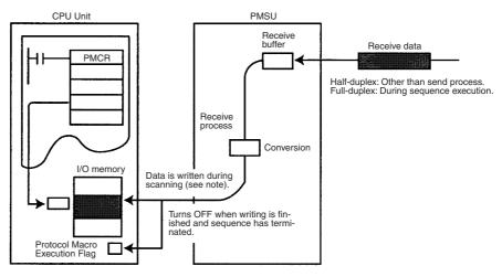
Note With the scan notification method, write timing will vary as shown below depending on the PMSU model.
