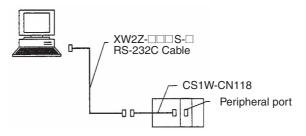
When combining the CS1W-CN118 with the RS-232C Cable, connections cannot be made using the **Toolbus**. Make connections using **Host Link** (SYSWAY).
