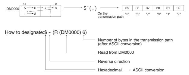
When converting the numeric data (ASCII data) from the external device into the hexadecimal data and receiving and writing it
