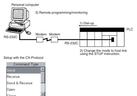
**Note** When set to modem control mode, the DTR signal will turn ON when the sequence is started and will turn OFF when the sequence ends. If the DTR signal is turned ON using the Open command under the modem control mode, the DTR signal will remain ON even after the sequence has ended.
