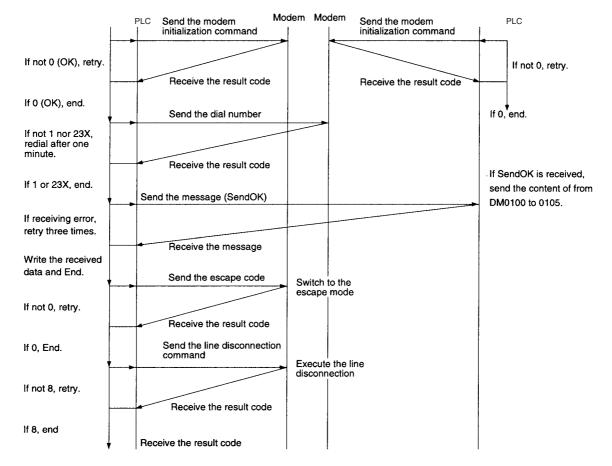
**Note** Information about the AT commands to be sent to the modem i.e. the initialization command, dial command, escape code sending, line disconnection command, etc. and result codes (response) is described in the manual of the modem in use. The modem used in this example is MD24FB10V (made by OMRON). AT commands and result codes supported by the modem are listed in the following tables.
