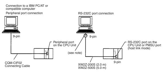
**Note** For IBM PC/AT or compatible computers, a conversion connector from D-sub 25P (female) to 9P (female) is required for the personal computer side connector.
