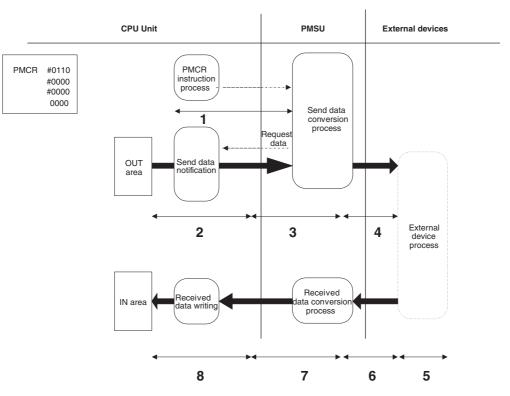
• Communications Response Performance Using the Link Word Area Illustrated below is the data flow when the link word area is used for the communications data storing area:
