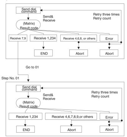
When configuring the steps, the enough consideration is necessary not only for the normal course (the process is completed in normal) but for the error course (the process is terminated by error). The error courses are often set to be aborted (intermittent process stop) all together. However, if the abort is set as the simple "other than normal course," the process stops there.
