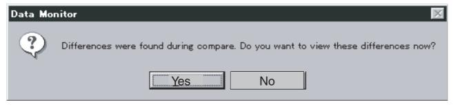
By left-clicking the **Yes** Button, the address of the data in the PLC will be displayed in parentheses.
