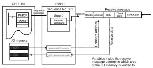
To designate which area of I/O memory is used for creating send messages and which area of I/O memory is used for storing receive messages, the following three methods can be used.
