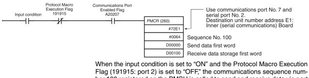
Flag (191915: port 2) is set to "OFF," the communications sequence number 100 registered on the PMSU is called to send and receive data via port 2 of the PMSU if the Communications Port Enabled Flag (A20207: internal logic port of the communications port No. 7 is used) is ON.
