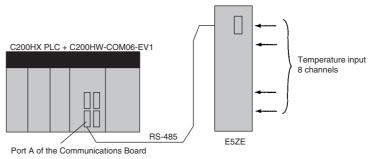
Eight points of measured temperature are assumed to be stored to DM101 to DM 116.
