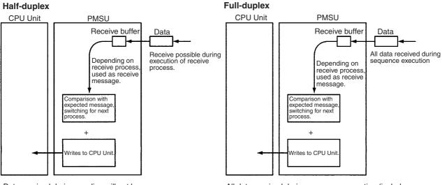
Data received during sending will not be used as receive data. Data received when not sending will be sent to the receive buffer. This data can be extracted using the receive process.
