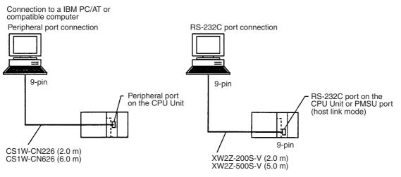
**Note** When using the RS-232C Cable to connect to a CPU Unit peripheral port, as shown below, use the CS1W-CN118.
