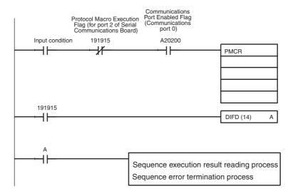
Example: The execution of the protocol Temperature Controller (E5 K Read System) Sequence No. 000 (read process value)
