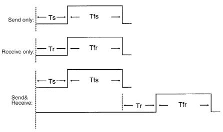
2. Be sure to set both the receive wait monitor time Tr and receive finish monitor time Tfr. With the CX-Protocol, it will not be possible to set just one of these.
