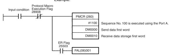
When the input condition is set to "ON" and the Protocol Macro Execution Flag (28908: port A) is set to "OFF," the communications sequence No. 100 registered on the PMSU will be called to send and receive data via port A of the PMSU.
