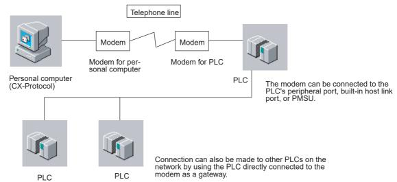
The setting procedures required to make connections to a remote PLC using modems are shown below.
