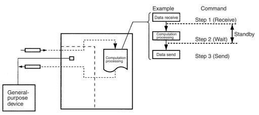
If used in combination with a matrix, it is possible to set up the system so that when certain data is received, the send/receive sequence will be put on standby and computational processing (e.g. data processing) will be performed at the CPU Unit before proceeding to the next communications process.
