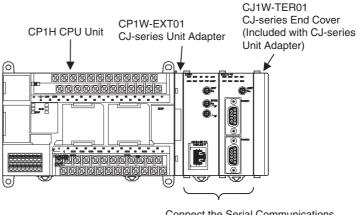
Connect the Serial Communications Unit to one of these.
