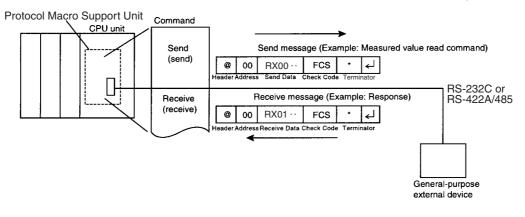
The sequence determines, according to the result of process, whether to send the same send message again (called retry) or execute the next process (reading process value from the Temperature Controller linked to another address, etc.), for example.
