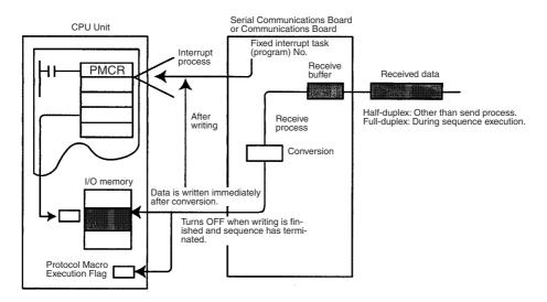
**Note** With the CS-series (Serial Communications Board), received data cannot be stored in the EM area using the interrupt notification. If this is attempted, a protocol macro syntax error (A42410) will occur.
