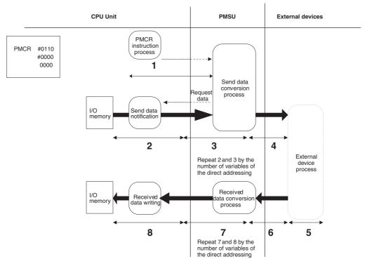
• Communications Response Time Using the Direct Addressing Illustrated below is the data flow when the direct addressing is used:
