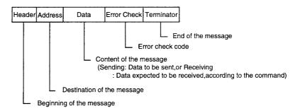
The check code and the terminator can be replaced with each other.
