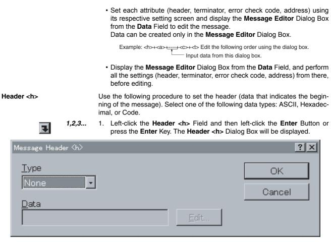
Select a header type from the **Type** drop-down list (refer to Code, ASCII, and Hexadecimal in the following section) and set the **Data** Field.
