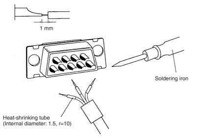
4. Move the heat-shrinking tube to the soldered section and shrink the tube by heating it.
