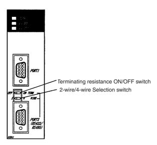
Setting the Serial Communications Unit Front rotary switch setting
