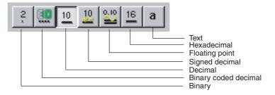
Note The default data display format in the PLC data table can be changed by selecting the new default data display format from the **Display** Tab in **Preferences** in the **Display** Menu.
