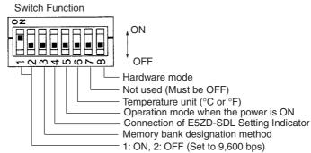
**Note** After changing the DIP switch settings, turn OFF and ON the power supply once.
