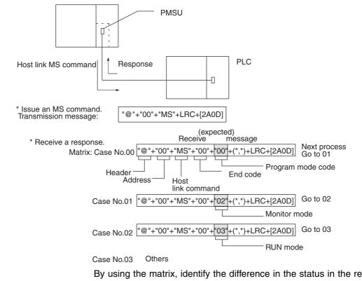
By using the matrix, identify the difference in the status in the response data (section in the above), and change over the process according to the mode of the PLC.
