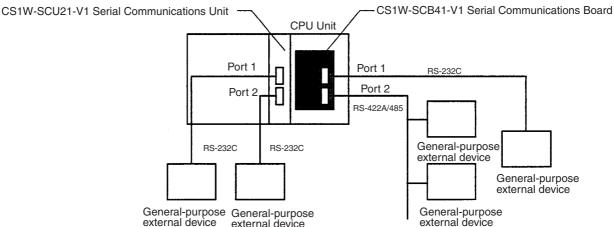
**Note** For connector pin arrangements and connection methods, refer to the CS/CJ Series Serial Communications Boards/Unit Operation Manual (W336) and other relevant manuals for general-purpose external devices.
