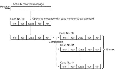
Therefore, if there are differences in message formats between cases because messages are opened up using the frame configuration of case number 00, comparison results for frames with a different message format from case number 00 will register a non-match, irrespective of the actually received message.
