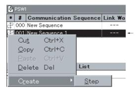
A new step is created after clicking the right mouse button or pressing the **Shift+F10** Keys to select the corresponding item in the popup menu. In this example, **Create/Step** is selected.
