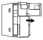
3. Insert the PMSU and slide it into the slit completely.
