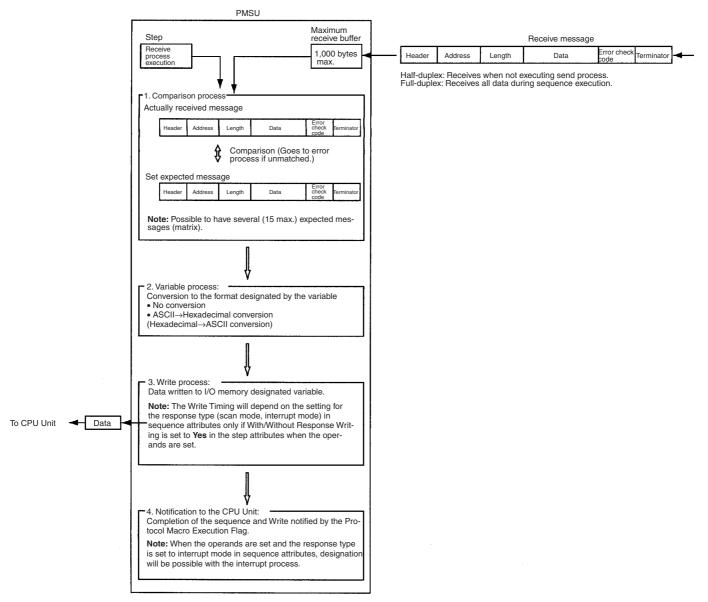
Send & Receive Process (Send & Receive Command) The receive (Receive) process will start approximately 60  $\mu$ s after the send process is completed.
