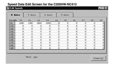
For the C500-NC113/211, values must be input within the range of 0 to 250000 (pps).
