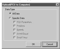
4. For the C200HW-NC113/213/413, specify the destination Position Control Unit unit number in the "Unit #" list box when selecting "Download (Computer to PCU)[D]" or specify the unit number of the source Position Control Unit in the "Unit #" list box when selecting "Upload (PCU to Computer)[U]." The default unit number displayed in the list box is the unit number specified in "Option(O)."
