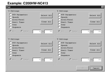
For two-axis control, the screen for the X and Y axes will be displayed. For one-axis control, the screen for the X axis alone will be displayed.
