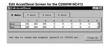
For the C200HW-NC113/213/413, input the acceleration data values and then press the Enter Key. The cursor will move to the deceleration data field.
