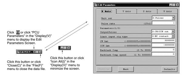
• Click the minimized data edit screen (icon) or on the left side of the minimized data edit screen to display the following menu.
