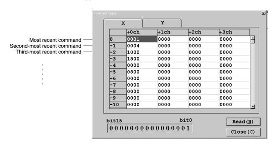
**Note** Command trace data will be lost when the Position Control Unit is turned off. Therefore, if you need see the trace data at system startup or when some trouble occurs, be sure to not turn off the power to the Position Control Unit.
