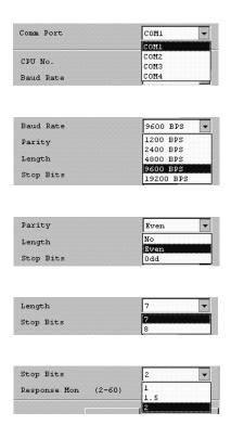
3. To change the CPU Unit's unit number and response monitoring time, input the new value directly. Unit numbers for CPU Units can be changed for the C200HW-NC113/213/413 PCUs only.
