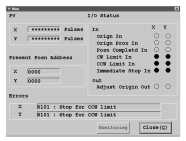
The latest error will be displayed. A filled circle (●) in the "I/O Status" box indicates that I/O activity is occurring. The present position and present position address will be displayed.
