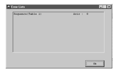
This error list indicates that the X-axis sequence data number 0 is invalid. After clicking "OK," check for invalid or missing data and correct the sequence data accordingly.
