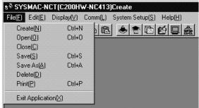
If shortcut keys are available for a function, the keys will be displayed to the right of the item. For example, the Ctrl + N Keys are allocated to "Create(N)." In this case, press the Ctrl + N Keys to create a new file. Furthermore, if the N Key is pressed while the menu is displayed, "Create(N)" will be selected.
