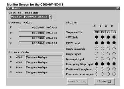
The present position of each axis will be displayed in the "Present Value" box. Error codes and details will be displayed in the "Error Code" box. The I/O status and sequence number for each axis will be displayed in the "Status" box. A filled circle ( ) indicates that I/O activity is occurring.
