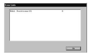
This error list indicates that the setting for the X axis of positioning action 0 is incorrect.
