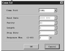
2. To change the communications port, baud rate, parity, data length, or stop bits, click "▼" and then select the desired setting. The baud rate, parity, data length, and stop bits can be changed for the C200HW-NC113/213/413 PCUs only.
