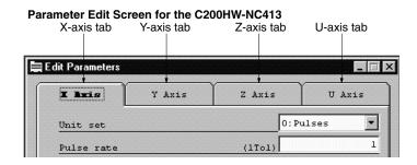
Clicking the Y-axis tab displays the Y-axis data edit screen. This also applies to the Z and U axes.
