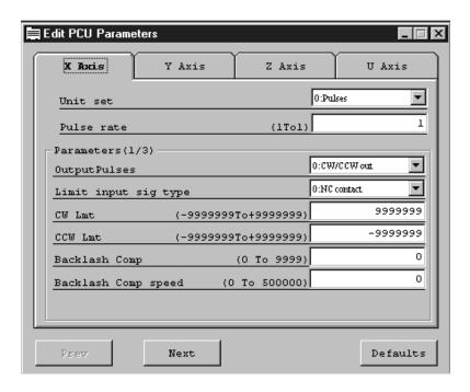
For the C200HW-NC113/213/413, three edit screens are used. For the C500-NC113/211, five edit screens are used. The previous page can be displayed by clicking "Previous" and the next page can be displayed by clicking "Next."
