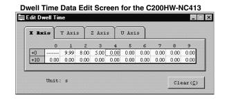
For the C500-NC113/211, values must be input within the range of 0 to 999 (x 10 ms).
