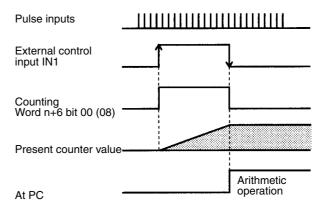
Offset phase inputs multiplied by 1 are input to the encoder. BCD data and external control input IN1 are used in the system.
