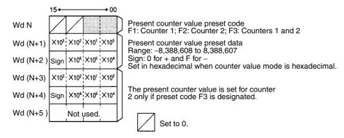
Transfer the present counter value in a block of data. If there is more than one block of transfer data, set the first block to the present counter value. The High-speed Counter Unit ignores the data in the succeeding blocks.
