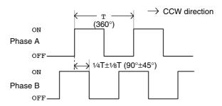
The output offset phase is  $90^{\circ}\pm45^{\circ}$ . Therefore, the greatest offset phase of the encoder is  $45^{\circ}$  (i.e.,  $90^{\circ}-45^{\circ}$ ).
