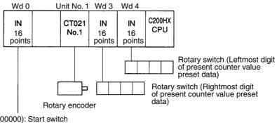
SW1 (00000): Start switch SW2 (00001): Data transfer switch
