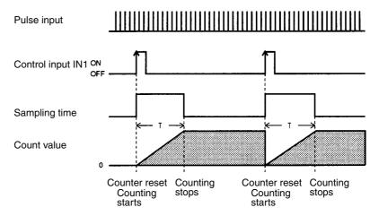
In this mode, the number of pulses will start counting from 0 when control input IN1 is turned ON and the timer for a preset sampling time will be turned ON at the same time. When the time is up, the High-speed Counter Unit will stop counting the number of pulses and keep the count value on hold.
