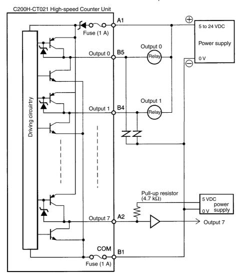
**Note** In the above connection example, the output power supply voltage must be higher than the load supply voltage, and if the external power supply is different from the load power supply, make sure that the external power supply voltage is the same as or higher than the load supply voltage.
