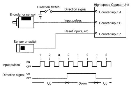
Counter input A is used as a direction signal. The High-speed Counter Unit will be in decrement operation when the direction signal is ON and in increment operation when the direction signal is OFF.
