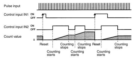
In this mode, the count value will be reset when control input IN1 is turned ON.
