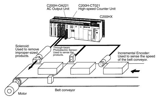
The High-speed Counter Unit counts the number of pulses that is input from the encoder while each product is passing between the emitter and receiver of the through-beam photoelectric sensor.
