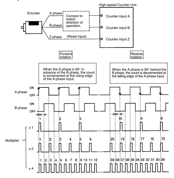
**Note** A counter can be reset with a Z-phase input from the encoder. Refer to *4-10 Counter Reset Conditions*.
