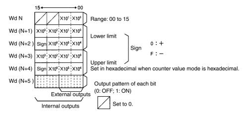
A block of data consists of a range number, upper limit, lower limit, and output pattern. Upper and lower limits must satisfy the following conditions.
