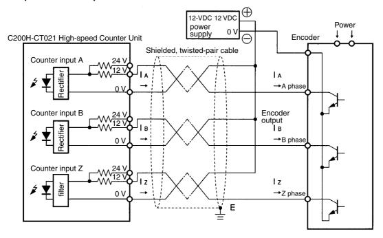
Wiring Example 2: 12-VDC Voltage-output (Sink Load) Encoder
