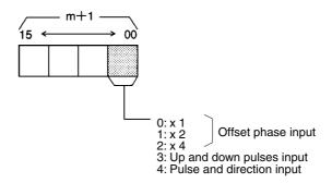
The type of input to counter 2 is set with word m+2.
