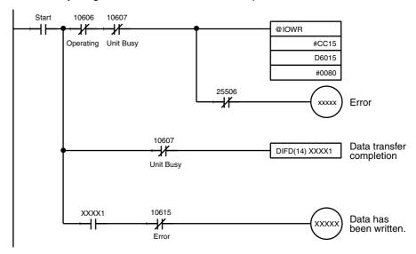
All the data has not been transferred when the IOWR instruction was completed. Use the Data Transfer Completion Flag or Unit Busy Flag to check the completion of data transfer.
