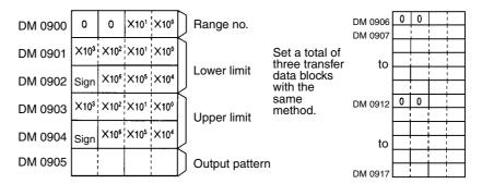
To transfer more than three transfer data blocks, store them in a different area, and move three data blocks to DM 0900 to DM 0917 to transfer each time. A total of three blocks of transfer data can be transferred at a time.
