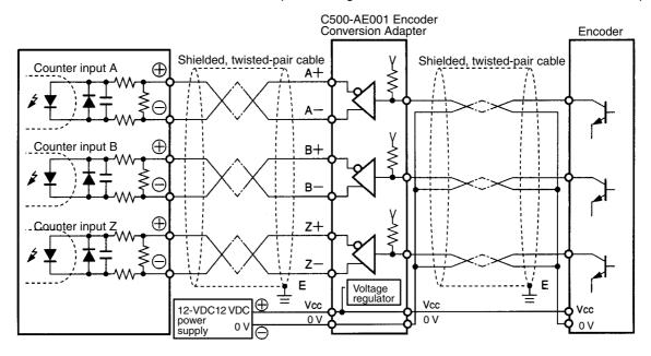
Note Connect the wires so that a counter input to the High-speed Counter Unit will be turned ON when an output from the encoder is turned ON.
