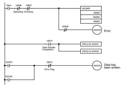
Bit 25506 will be turned ON when the IOWR instruction is executed with no errors and turned OFF if an error results.
