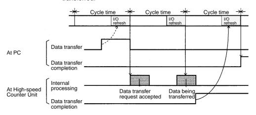
**Note** When the High-speed Counter Unit is mounted to a Slave Rack, there may be a data transfer delay between the Master and the Slave. Refer to *C200H PCs Operation Manual* for details.
