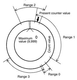
The example below uses the following lower and upper limits with the outputs to be turned ON.
