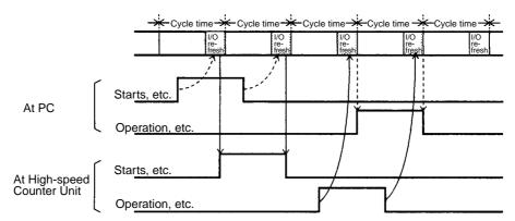
The data transfer completion bit will be turned ON or OFF whenever data is transferred.
