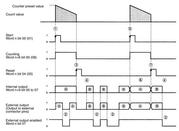
In the above timing chart, (A) indicates normal outputs and (B) indicates forced external outputs provided that the forced external output function is enabled.
