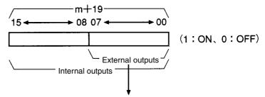
To output pins 0 to 7 of the external connector.
