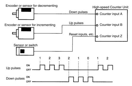
The High-speed Counter Unit counts up and down pulse inputs when the pulses are turned ON.
