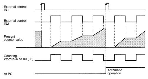
Offset phase inputs multiplied by 1 are input to the encoder. BCD data is used in the system.
