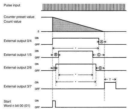
External outputs 0 to 3 are for counter 1 and external outputs 4 to 7 are for counter 2.
