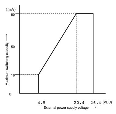
**Note** The output current must not exceed 0.5 A per common (i.e., eight points), otherwise the built-in fuse will blow out. The built-in fuse cannot be replaced by the user.
