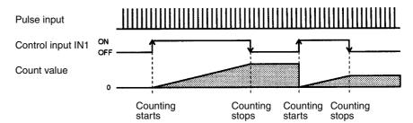
In this mode, the present counter value will start counting from 0 when control input IN1 is turned ON and stops counting the present counter value at the falling edge of IN1. The count value will be kept on hold until control input IN1 is ON again.
