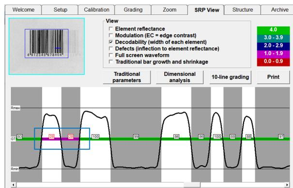
Bars and spaces with widths deviating from the criteria are given low grades.
