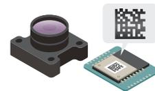
Barcodes are printed on modules including onboard chips and sensors to make it possible to trace individual items.
