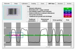
Bars and spaces with widths deviating from the criteria are given low grades. (Highlighted in blue)
