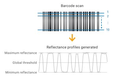
Assume that there is one defect in a barcode. Of ten scan attempts, the reflectance of an attempt that scans the defect will change from that of the others. Observation of the change in reflectance leads to detection of the print quality problem, and results in a lower grade.
