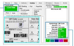
An overall grade is determined from the verification results of verification items Quality is graded through verification items specified in international standards
