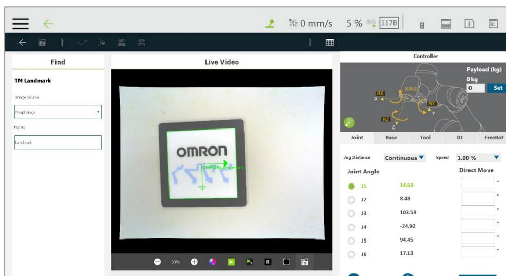
Figure 10: Landmark Alignment (1/2)
