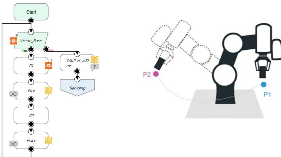
Figure 5: The Flow of Pick and Place
