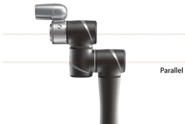
When the fourth and sixth joint are nearly parallel, is the robot is about to entering the Wrist Singularity Point in Space.
