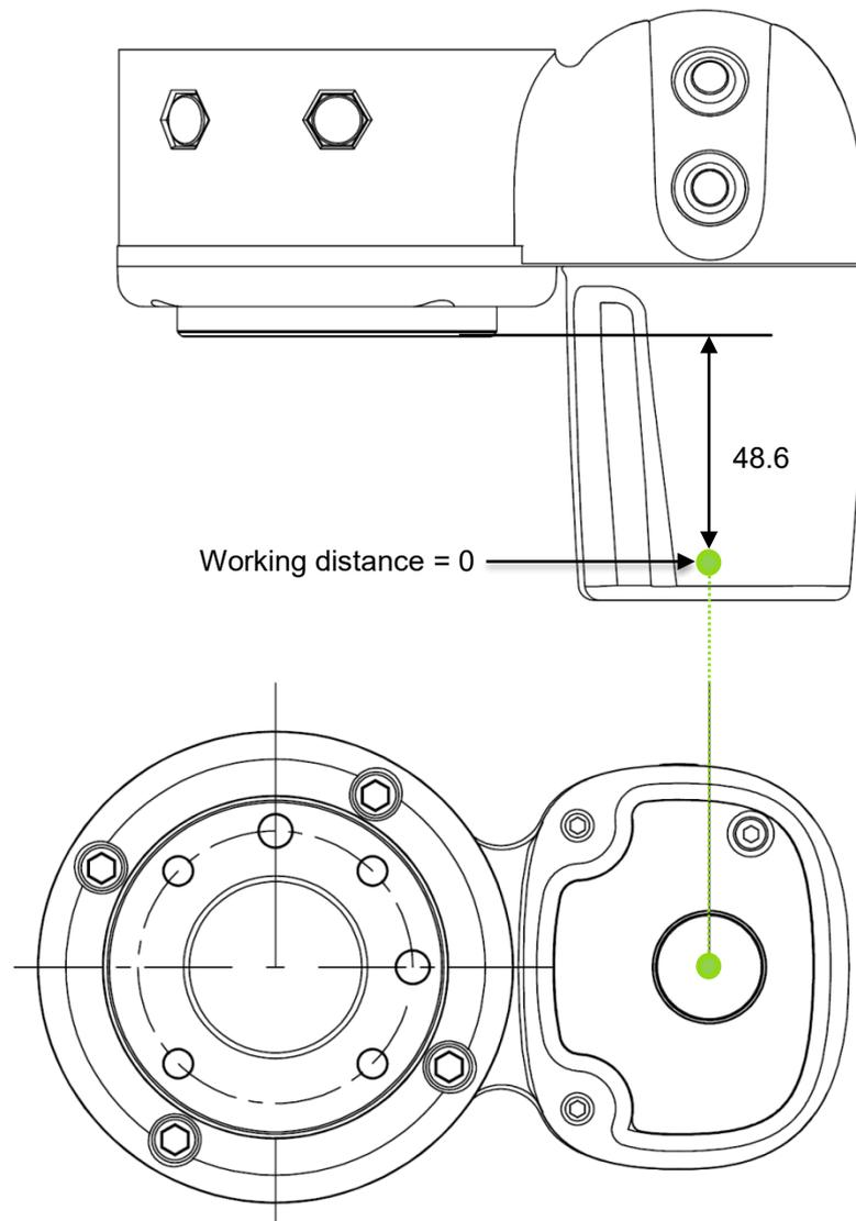
The relation between the working distance and the field of view is listed below,
