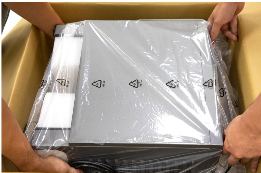
The control box should be carried by at least two people. One should hold on to the control box handles, while the other should carry the foot stands. Before handling, the cable of the robot stick should not be pulled to avoid any performance degradation.
