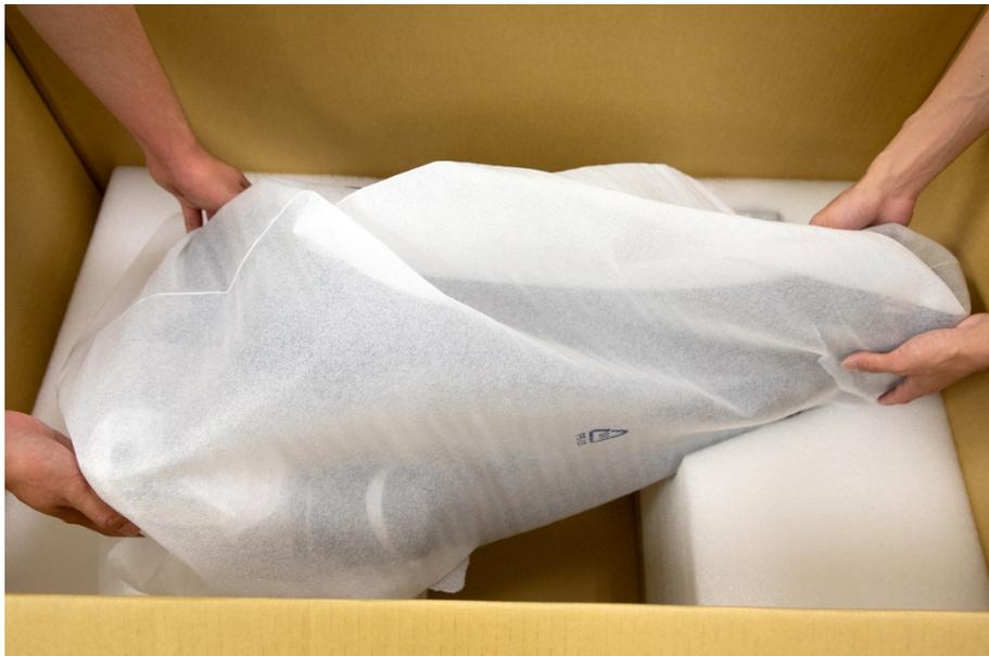
The Robot Arm itself should be handled with at least two people. One person should carry the Lower arm and Upper arm, and the other should hold on to the position between the base and 1<sup>st</sup> Joint as well as the 6<sup>th</sup> Joint. Before the Robot Base is fastened with screws tightly, the Robot Arm should always be supported to avoid tipping.
