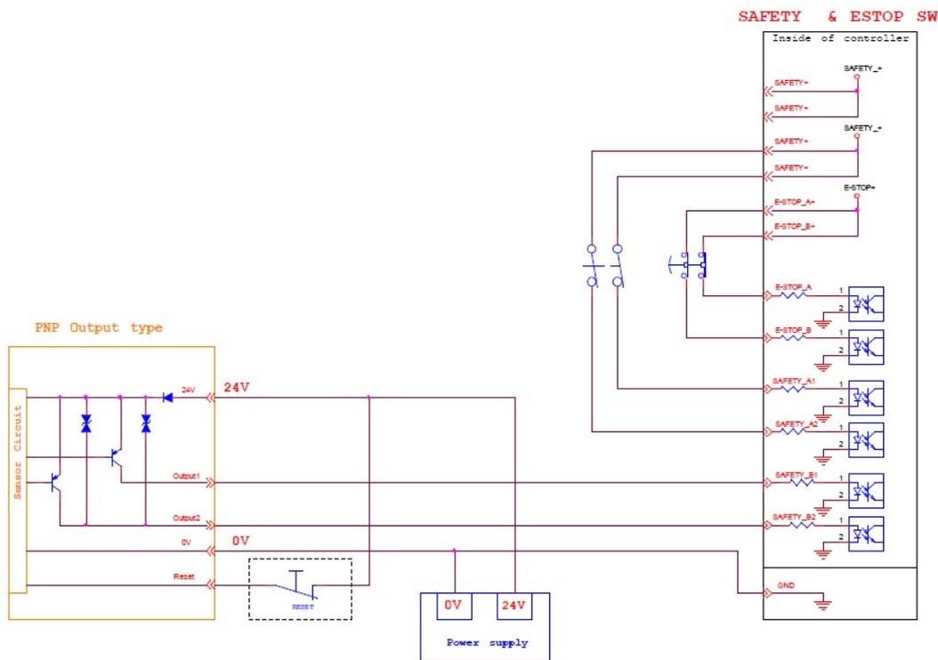
The wiring diagram shows the example of PNP output type safety device.
