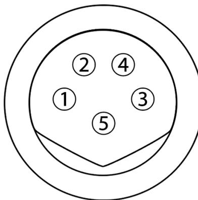
5-pin analog I/O connector of Robot
