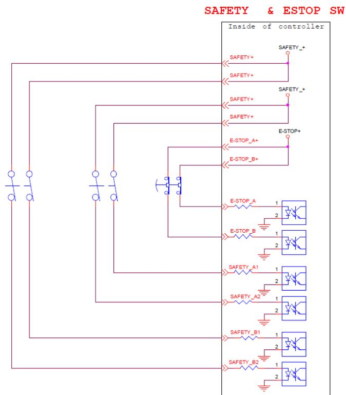
The wiring diagram shows the example of switch type safety device.
