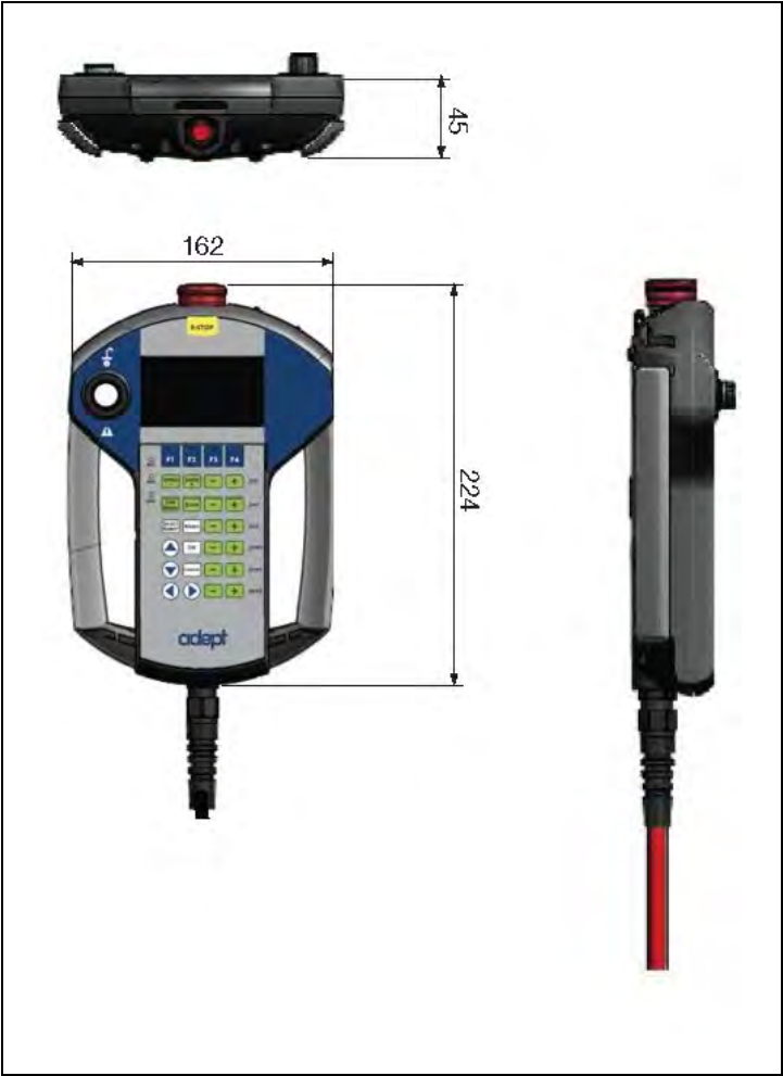
Figure 5-3. T20 Pendant Dimensions (Units in mm)
