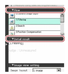
2. When displaying both the flow and detailed results, you can change the size of the Display area of the flow and detailed results by dragging [Detail result].
