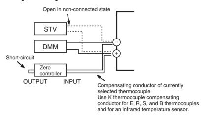
Disconnect the STV to enable the thermocouple of the cold junction compensator. When doing this, be sure to disconnect the wiring on the STV side.
