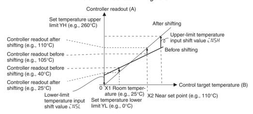
Figure 3 Illustration of 2-Point Shift
