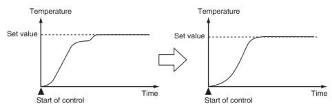
• When the manipulated variable (MV) is saturated, the amount of overshooting may be somewhat higher in comparison to PID control based on AT or ST in normal mode.
