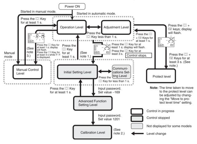
**Note** (1) Moves to operation level by software reset.
