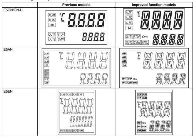
Basically, the Controllers are upwardly compatible. The terminal arrangement, terminal sizes, and depth for panel mounting have not been changed. Changes are listed in the following tables. For details, refer to the pages given for specific items in the index.
