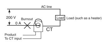
The heater power supply provides 5 A when the current is normal, and 0 A when there is a burnout, so the heater burnout detection current is calculated as follows:
