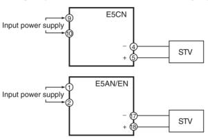
• Operation Set the STV output to the voltage or current equivalent to the check value.
