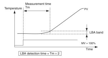
Loop Break Alarm Section 4-12
