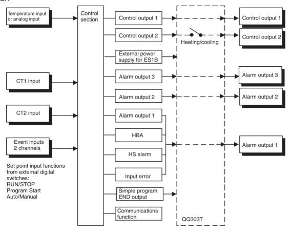
**Note** Functions can be assigned individually for each output by changing the set values for the control output 1 assignment, the alarm 1 assignment, the alarm 2 assignment, and the alarm 3 assignment in the advanced function setting level.
