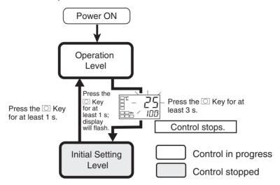
To move from the operation level to the initial setting level, press the  $\bigcirc$  key for at least three seconds with any parameter displayed except for the "auto/manual switch" parameter.
