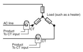
3. V connecting lines: Refer to the following diagram for CT installation positions.
