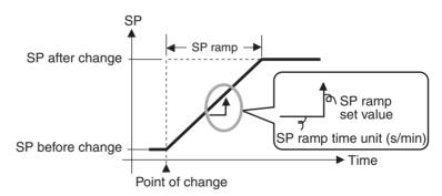
The rate of change during SP ramp is specified using the "SP ramp set value" and "SP ramp time unit" parameters. The "SP ramp set value" parameter is set to OFF by default, i.e., the SP ramp function is disabled.
