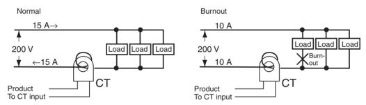
The heater power supply provides 15 A when the current is normal, and 10 A when there is a burnout, so the heater burnout detection current is calculated as follows:
