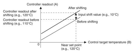
Figure 2 Illustration of 1-Point Shift
