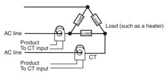
2. Star connecting lines: Refer to the following diagram for CT installation positions.
