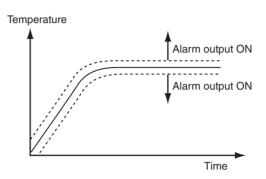
Alarm SP Selection = Target SP (Alarm Type: 1 (Upper/Lower Limits))
