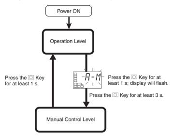
To move from the operation level to the manual control level, press the  $\square$  key for at least three seconds with the "auto/manual switch" parameter displayed.
