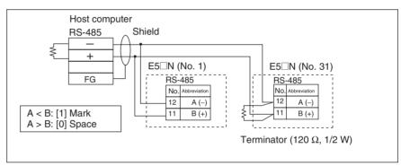
The RS-485 connection can be either one-to-one or one-to-N. A maximum of 32 Units (including the host computer) can be connected in one-to-N systems. The maximum total cable length is 500 m. Use AWG24 (cross-sectional area: 0.205 mm²) to AWG14 (cross-sectional area: 2.081 mm²) shielded twisted-pair cable.
