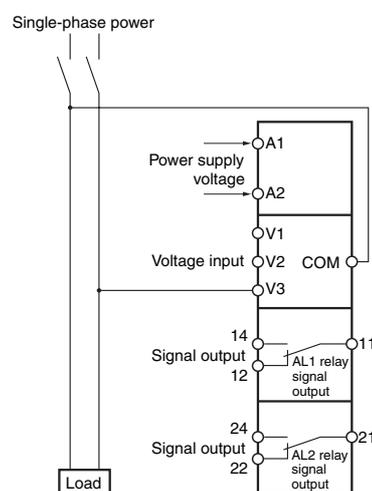
**Note:** There is no polarity when a DC current input used.
