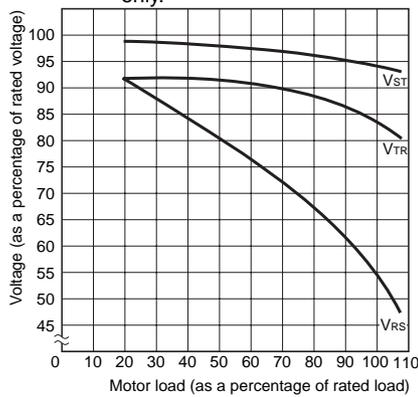
**Note:** For phase loss of phase R. V<sub>st</sub>, V<sub>tr</sub>, and V<sub>rs</sub> indicate the motor terminal voltage at phase loss.
