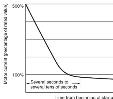
For a motor with a rating of 5 A, the startup current will be approximately 30 A. The startup current will exceed the overload capacity (rating: 150% for 1 s) of the K8AB-AS1 and K8AB-AS2 and result in failure of the Relay. To monitor the motor load, use the K8AB-AS3. (Overload capacity: 120% of rating for continuous load, 200% of rating for 30 s, and 600% of rating for 1 s). The K8AB-AS3 has a large input range. Pass the conductors multiple times through the special CT.
