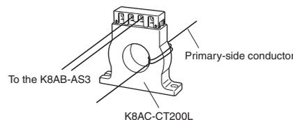
**Concept behind Passing Conductor through the CT When Using the K8AB-AS3**
