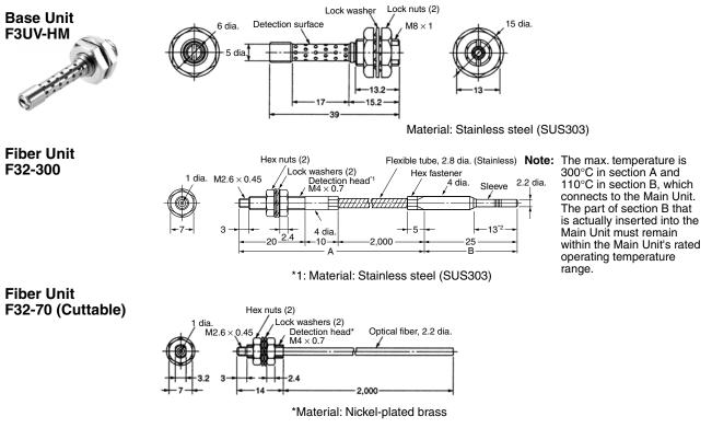
Note: The "cuttable" Fiber Units can be cut to length. Units that are not marked "cuttable" cannot be cut to length.
