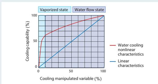
+ Water-cooling output adjustment function
