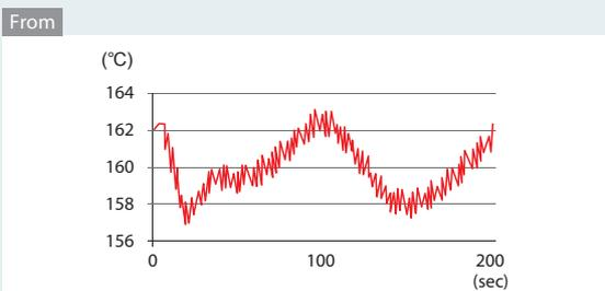
When a temperature sensor for a packaging machines is used, there is sometimes periodic temperature variation generated when there is a marked effect from the heat on the packaging materials side.
