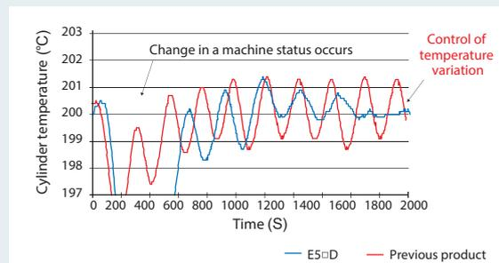
\* Data measured by OMRON on a water-cooled twin screw extrusion molding machine.
