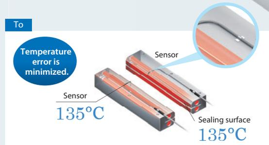
The installation position of the temperature sensor for packaging machines has been brought closer to the sealing surface to bring the temperature of the sensor closer to the temperature of the sealing surface. This minimizes the effects from variation in the surface temperature of the packaging materials.
