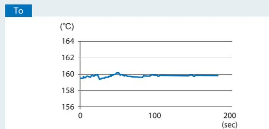
When the automatic filter adjustment function of the E5□D /NX-TC is used, this periodic temperature variation is suppressed automatically. It becomes possible to perform stable temperature control.
