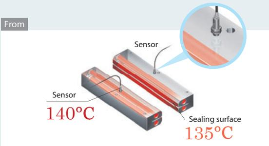
On a conventional sealing machine, temperature sensors can often be located too far away from the sealing surface, so a difference occurred between the temperature of the sealing surface and the temperature that was actually being controlled. This temperature difference and resulting sealing failures increase as the packaging speed increases.
