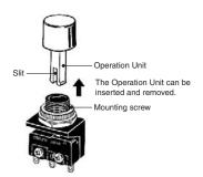
Tighten the hexagonal nut while securing the Switch by holding it with your fingers. Tighten the hexagonal nut with a torque of 0.49 to 0.98 N·m.
