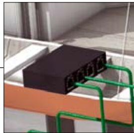
One switch as MRP manager controls the PROFINET-compliant redundant ring.
